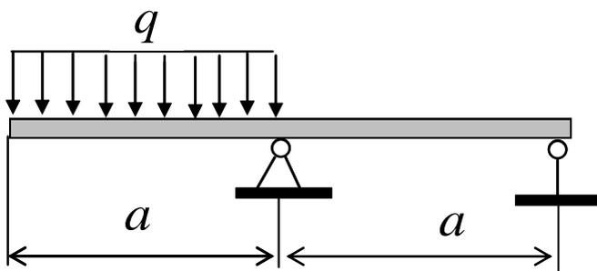
$$a = 1 \text{ m}; \quad q = 10 \text{ кН/м.}$$
