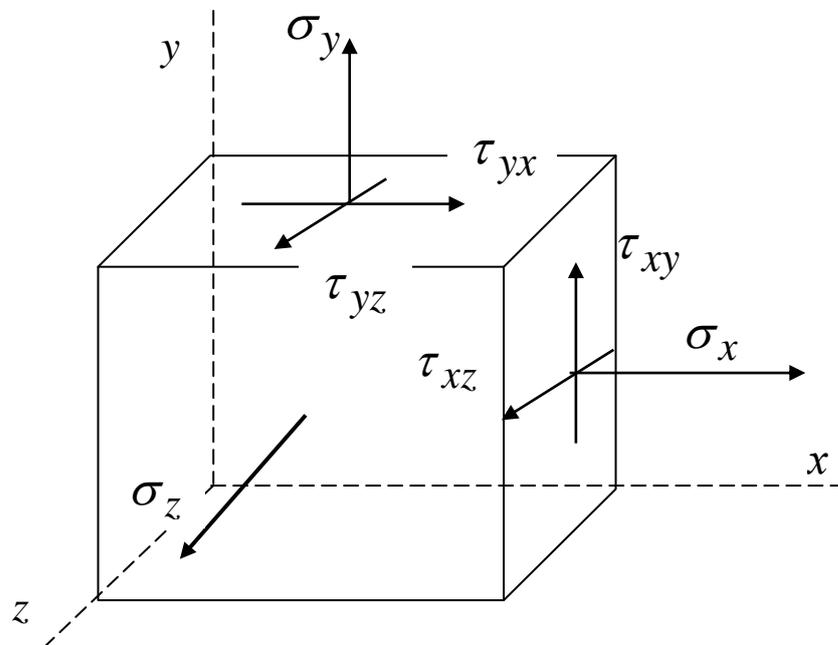
$$\sigma_{max/min} = \frac{(\sigma_x + \sigma_y)}{2} \pm \sqrt{\left(\frac{\sigma_x - \sigma_y}{2}\right)^2 + \tau_{xy}^2}$$
